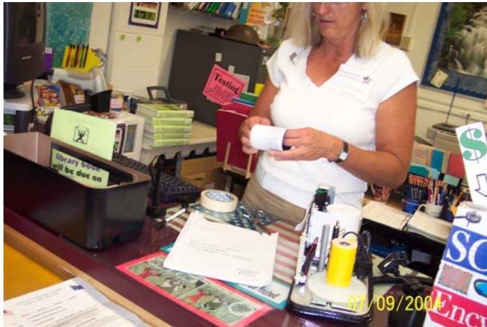
Figure 3: Poll Worker attempting to fix a jammed VVPAT printer. [11]
